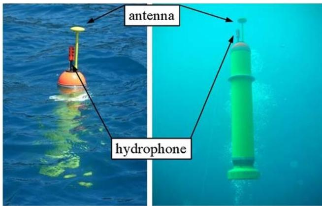
▲ **Figure 1.** Picture of a Mobile Earthquakes Recording in Marine Areas by Independent Divers (MERMAID) float (Hello *et al.*, 2011). The color version of this figure is available only in the electronic edition.
