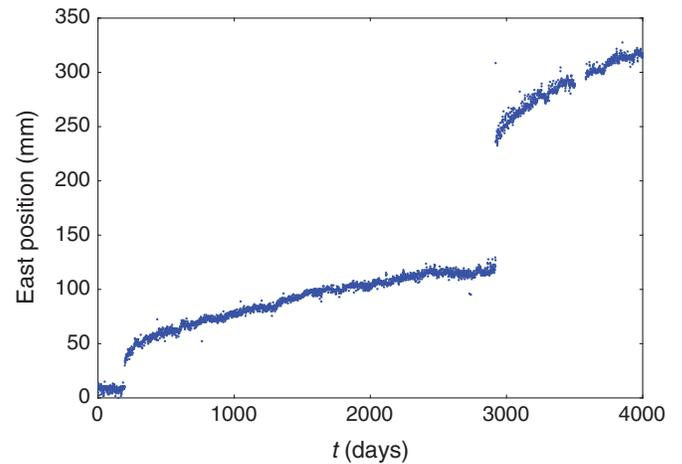
▲ **Figure 2.** Example ~11-year GNSS time series from east component of GEONET GNSS 020893 in Japan. The large upward jumps in the time series represent the coseismic displacements from large earthquakes. The nonlinear curvature following the two coseismic jumps indicates rapid postseismic deformation.
